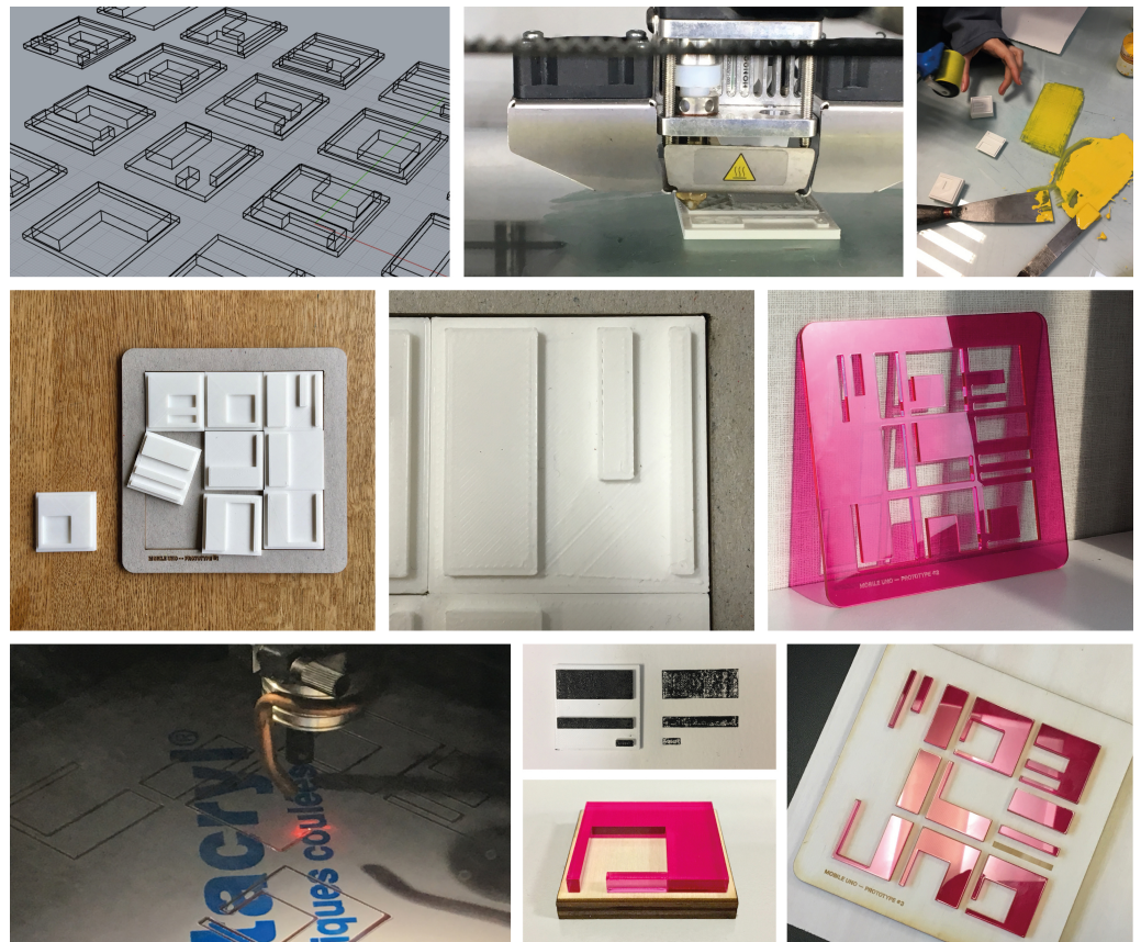
[Mobile Uno] FROM LEFT TO RIGHT, FROM TOP TO BOTTOM. Process of design and production, and final results. 3D printed titles for letterpress printing. Plexiglas stencil. Study of mixed materials: wood and plexiglass.
